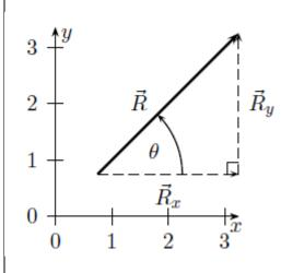
> When resolving into components that are parallel to the xand y-axes we are always dealing with a right-angled triangle.
